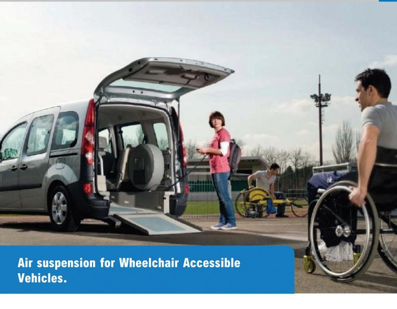
A major advantage of our air suspension is that it can lower your vehicle towards the floor to aid entry and exit. This is especially useful for wheelchair users as it significantly reduces ramp angles. An additional advantage is that a shorter ramp can be used, thereby reducing weight and improving the rear view of the driver.
