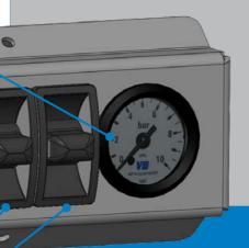
Every VB-SemiAir comfort system contains a manometer, a high/low switch and a compressor with high load-bearing capacity. The high/low switch enables you to raise or lower the ride height of your vehicle and allows you to pump the air spring in the best possible way. The manometer provides an accurate indication of the pressure in bar inside the air springs.
